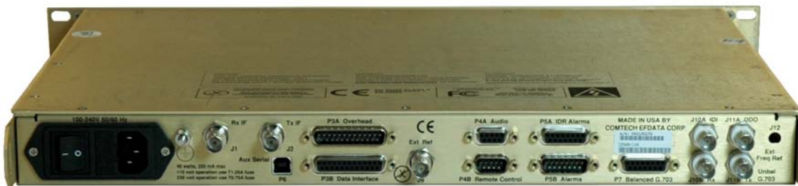
CDM-600 Satellite Modem Back Panel
